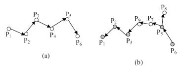
Figure 6. Propagation in a MANET: a) forward phase, b) backward phase.
